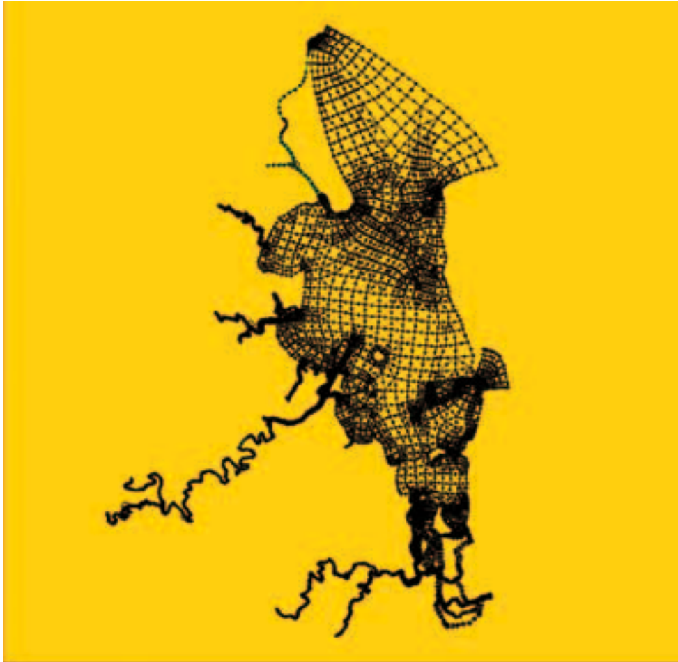
Figure 8.7c: Revised RWQM2 Mesh of the Airport Surrounds showing Bathymetric Data.
