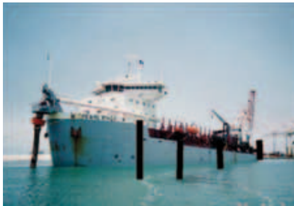
Figure 9.2e: Large TSHD and mooring piles, (Source: figure courtesy of Baggerman Associates).
