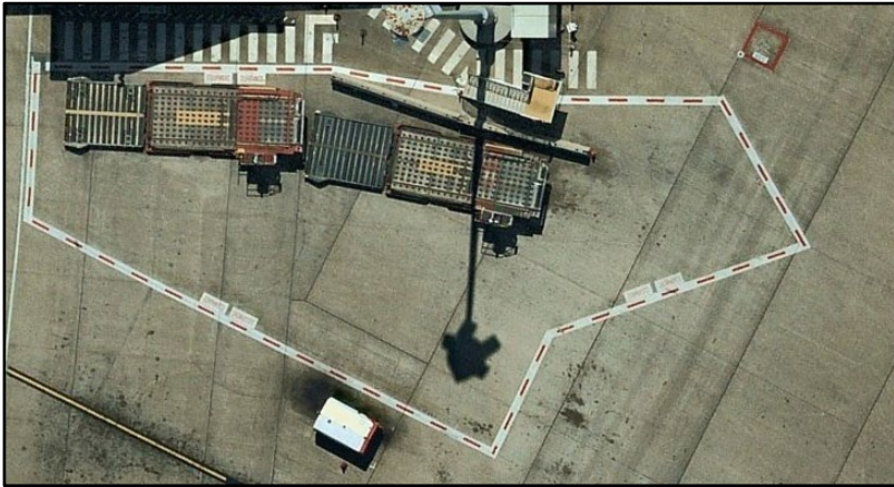
Figure 20 Single Broken Red Line - Staging / Clearance
